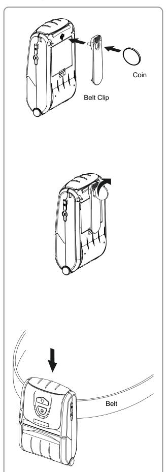
1) Insert the screw of the belt clip to the belt clip mounting hole.
