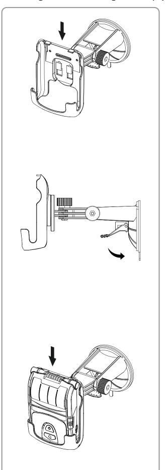
1) Assemble the vehicle holding cradle to the mount.
