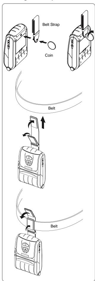
1) Insert the belt strap screw into the belt strap hole.
