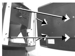
After matching the stand and monitor, push the stand to the arrowed direction as show in the right picture. At this time, turn the monitor to the normal position and plug the power then it can start to use.
