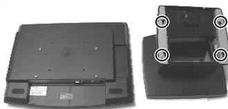
Please find the four holes in the top of stand. Take the stand and align these four matching holes to the four matching pegs which are in the back on monitor.
