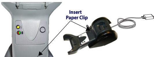
Figure 5. Disconnecting the Cable
