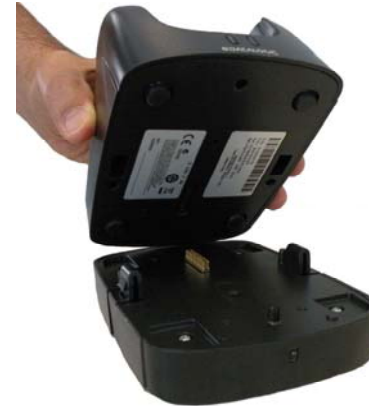
Figure 2 – Single Slot Dock Ethernet Module Installation
