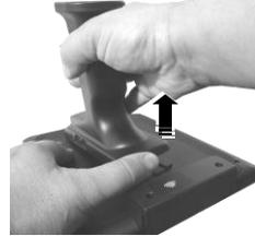
3. Align the hand strap cover with the grooves on the rear side of the table.
