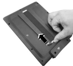
6. Fasten the hand strap cover onto the tablet using a screw.
