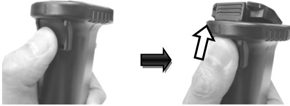
2. To replace the existing battery, gently push the metal clip outwards to release the battery. If you are installing the battery for the first time, please skip to the next step.
