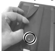
2. Slide the hand strap cover down in the direction indicated by the arrow.
