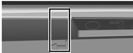
4. To check how much battery capacity remains in PG-200 pistol grip, press the battery capacity checking button on the pistol grip to show the current battery capacity level through the LED indicator.
