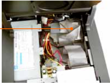
FIGURE 2-12: FOLDING THE IDE CABLES
