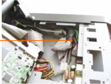
FIGURE 2-11: TUCKING THE IDE CABLES
