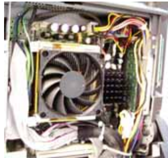
FIGURE 2-7: MAIN BOARD WITH CPU, FAN AND RAM INSTALLED
